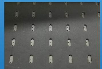
9. The belt adopts a fully automatic correction scheme and a reasonable suction holes design, which firmly absorbs the material during the transportation of the material, so that the quality of the printing is higher.
