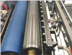
Closed doctor blade chamber / Coating by anilox roller
