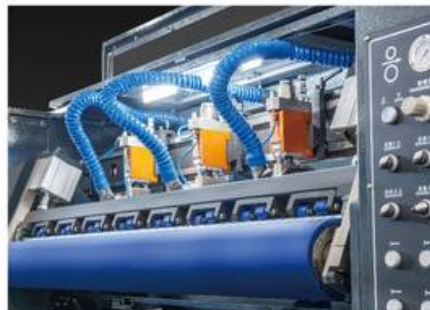
自动防爆辊反曲 (选配) CRACK PREVENTION ROLLER WITH AUTO ANTI CURVE (OPTIONAL)
