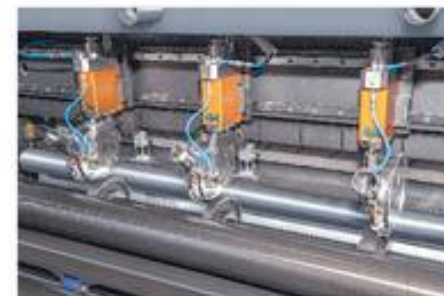
气动纵刀, 三条分条刀可供修边及对割 Three sets of slitting knife are used for trimming and middle slitting
