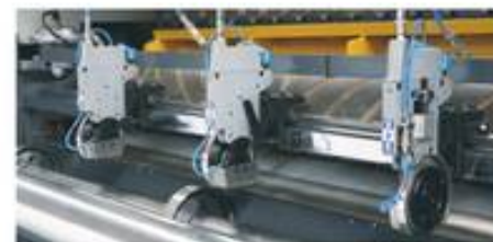
三组分条刀可供修边及对割 (选配) Three sets of slitting knives are used for trimming and middle slitting (optional)
