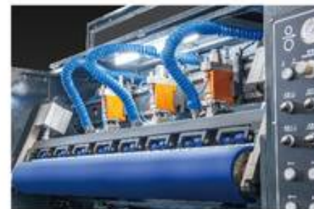
自动防爆辊反曲 (选配) Crack prevention roller with auto anti curve (optional)
