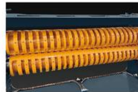
嵌入式螺旋双刀 (发明专利) Embedded double helix knife (invention patent)
