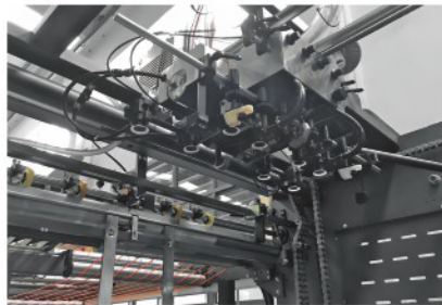
Four sucking and four forwarding high speed feeder
