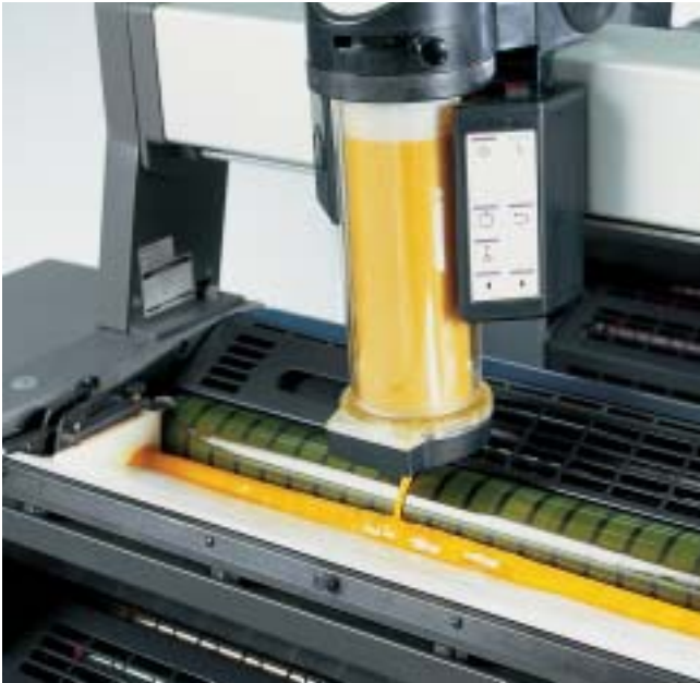
InkLine ensures automatic, cost-saving ink fountain replenishment.
