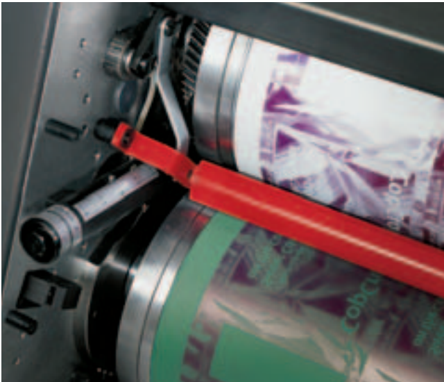
Helically toothed gears and bearer-on-bearer pressure ensure excellent print quality.
