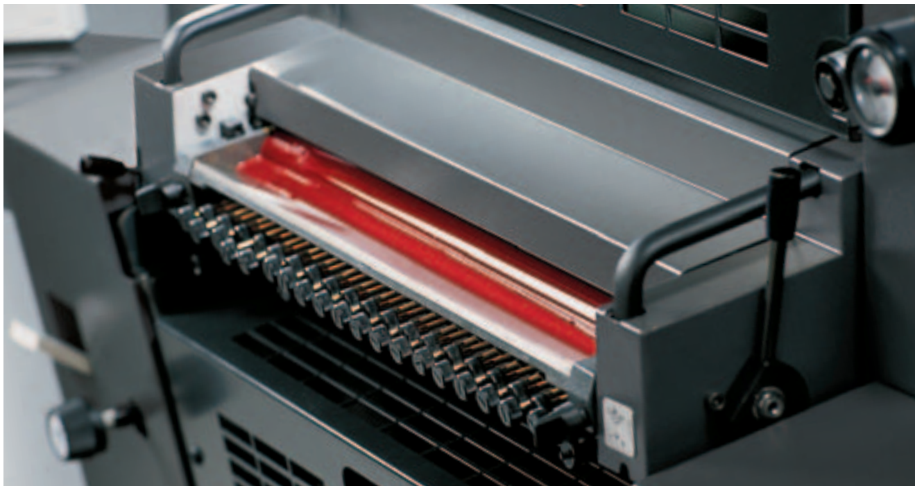
Mobile inking unit for numbering adds versatility.
