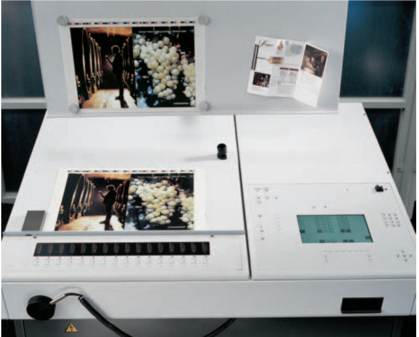
ClassicCenter – the ergonomic workstation for ink and register.
