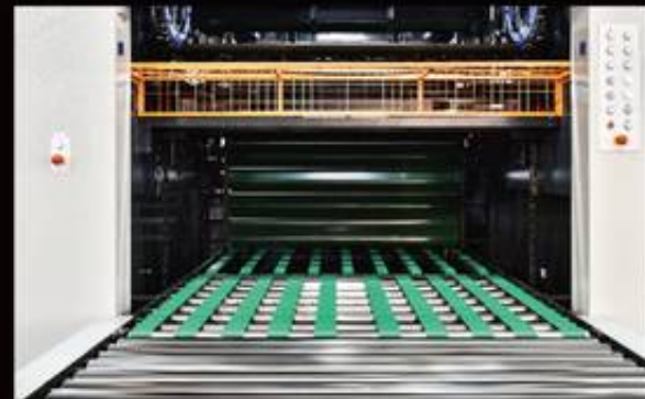
Batch conveying delivery unit
