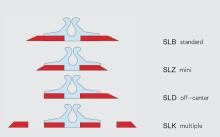
Mini model is used where the creasing rule is very close to cutting rule
