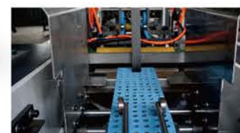
VACUUM SUCKING & SERVO MOTOR FEEDING
