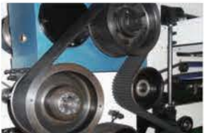
Torque limiter, intermittent segmentation
